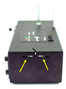
When the thread cutter becomes dull, the blade can be adjusted to provide a fresh, sharp cutting surface. Using a 2mm allen wrench, loosen the two screws holding the cutting blade. Do NOT completely remove the screws! Slide the blade either to the left or the right. Re-tighten the screws to hold the blade firmly in place.
