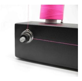
To adjust the tension of the Professional Bobbin Winder, turn the black knob clockwise to increase tension or counter-clockwise to decrease tension.
