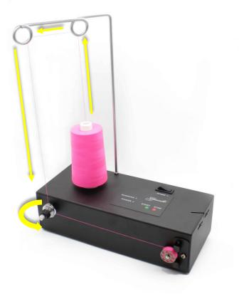
Now, it's time to wind bobbins! First, slide the thread through one of the holes in an empty bobbin from the inside toward the outside. Next, while holding the thread, place the empty bobbin on the motor spindle and push all the way on.
