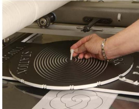
By using each of the sides you are able to stitch various sizes of ovals, wavy or straight lines, circles and rounded corner squares.
