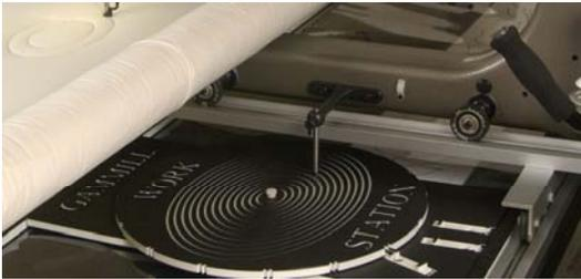
The two parallel white sliders are used to obtain precise positions along the table in increments of one groove. Only one of the sliders is used at a time to achieve the one groove increments.
