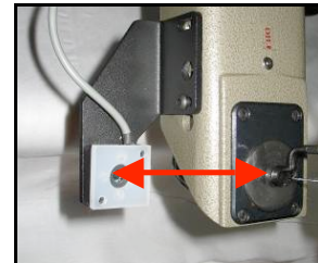
Camera eye is 3 ½" to the left of the needle.
