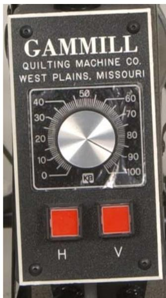
The dial can be turned from 0 to 100% of the motor speed. The speed can be changed as you stitch if needed. The red square buttons marked **H** and **V** are for the horizontal and vertical channel locks respectively.
