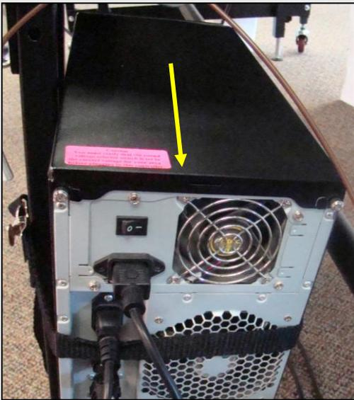
**STEP 2:** Remove the lid by sliding it towards the back of the Controller. A slight downward force may be necessary.
