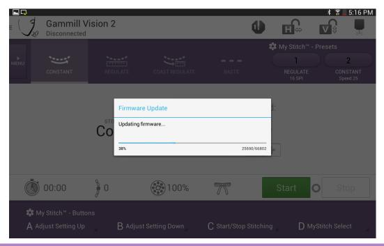
ONCE THE UPDATE IS COMPLETE, THE BLUETOOTH CONTROL BOARD WILL AUTOMATICALLY RESET AND RECONNECT TO THE APPLICATION.
