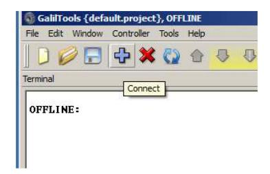
**STEP 25:** Individually try each COM port (ie COM1, COM2, etc) and press Connect until a connection is made.
