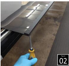
STEP 3: Using a #2 Philips head screwdriver, remove all screws on the bottom side of the tabletop. (See Figure 02)
